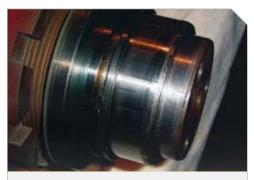
FIGURE 4 - NSK #NU326 280mm oil-lubricated bearing after more than 80,000km of high-speed service.
