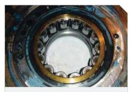
FIGURE 3 - Inner race of same NH219 greased bearing after disassembly.
