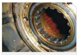
FIGURE 2 - NSK #NH219 170mm greased bearing after more than 80,000km of high-speed service.
