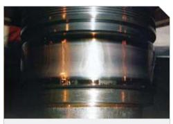
$\ensuremath{\textit{FIGURE 5}}$  - Inner race of same NU326 greased bearing after disassembly.
